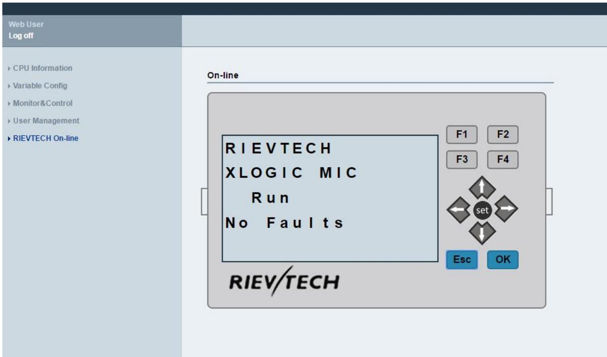
The CPU only can get a trigger from the virtual keys, it cannot get a continuous signal, that means if you press the OK key for 3 seconds, the CPU cannot know it pressed down 3 seconds, it only get a trigger signal. So if you want to realize the press ok key for 3 seconds to change the parameters in the text message on the hardware, you need press the "set" key on the virtual panel.
