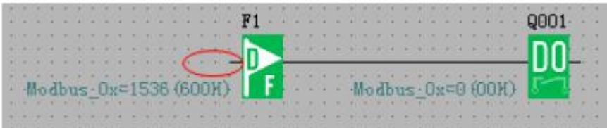
When the input pin of digital flag variable F is not connected, you can change the status of variable F.
