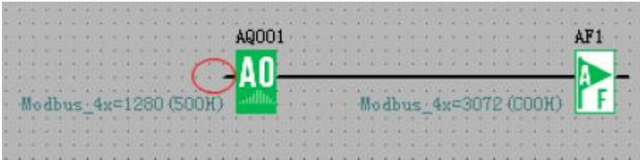
When the input pin of analog output block AQ is not connected, you can change the value of variable AQ.
